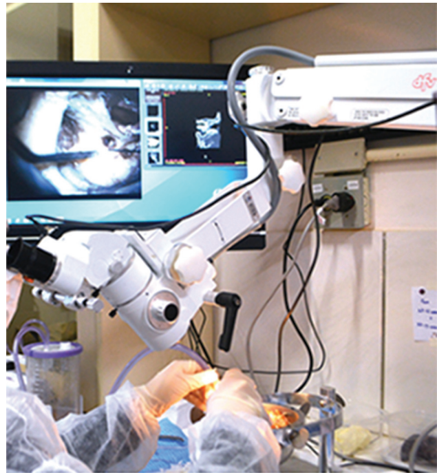
Fig. 3 Workstation with a MC-M22 microscope (DF Vasconcellos Ltda.) and a computerized video system linked with a monitor. Screen shows simultaneously the video of dissection transmitted in real time from microscope next to a software window with CT images of the temporal bone being dissected. Abbreviation: CT, computed tomography
